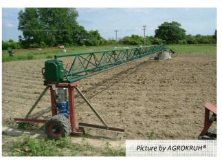
manual works etc. The mechanism is deigned for maximum of 12kWh electrical input for full operation of all machinery, but normally it is only about 5 kWh. Different implements and tools used in vegetable cultivation can be attached to the frame and are moved on the spiral. The frame can be easily moved to other circle after work is completed at a previous one. For the whole farm of 15 circles it is optimal to have 5 frames which can work simultaneously on different circles.
